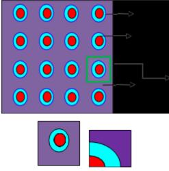
Figure 1.(a)Uniform distribution of spherical particles in matrix. (b)Isolated Unitcell and (c)one eigthmodel
