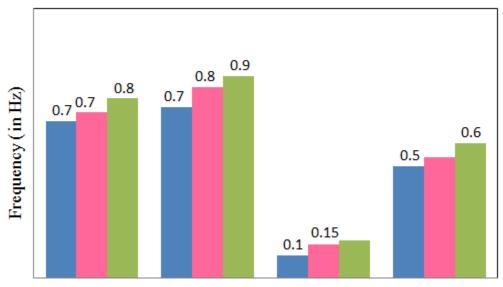
Fig 12.Result graph of natural frequency of 1,2,3 wt% CNT reinforced composite for all end conditions.
