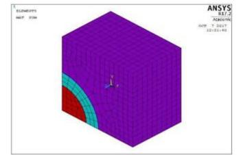
FIG.3 Converged mesh model of SWCNTs reinforced composite at 1 wt% of SWCNT.
